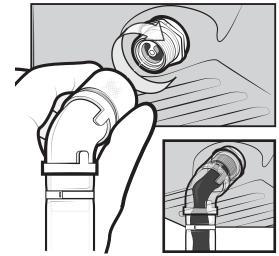
THREAD ON THE DRAINER TO RELEASE THE VALVE, AND TO ALLOW THE WASTE OIL TO FLOW FREELY.
