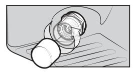
REMOVE THE DUST CAP FROM THE BASE OF THE PLUG.
