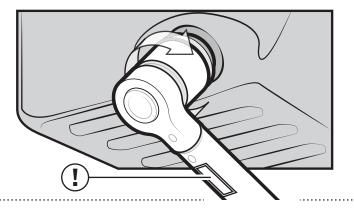
USE A TORQUE WRENCH TO TIGHTEN THE NO-SPILL™ PLUG TO THE TORQUE SPECIFIED ON THE PRODUCT CONTAINER.
