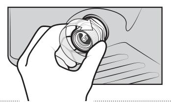
THREAD IN THE NO-SPILL™ DRAIN PLUG BY HAND UNTIL SLIGHTLY SNUG.
